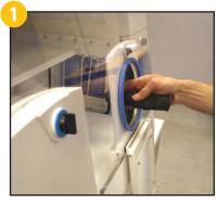
Roll a replacement membrane and insert into the workstation through the membrane that is not being replaced.
