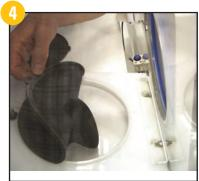
Carefully peel the existing membrane out of the retaining slot in the membrane carrier.
