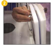
Reach through the workstation to the back of the membrane that is to be replaced.
